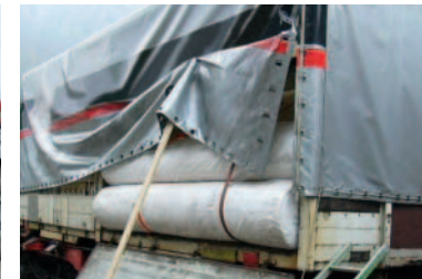
load slippage due to inadequate securing of freight
