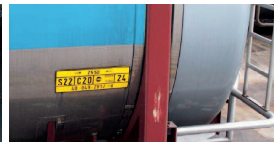
tank container with UIC identification code
