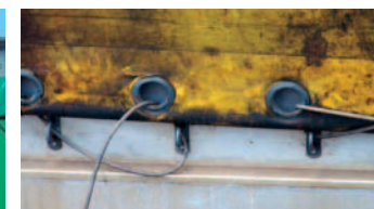
unacceptable securing of tarpaulin with TIR cable
