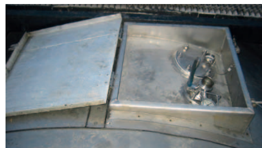
protection cap for armatures not closed
