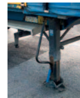
loose support leg crank
