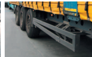
bent side underride guard
