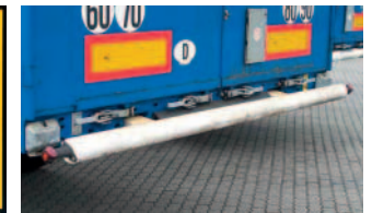
upward retracted rear underride guard
