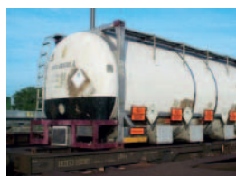
4-chamber tank container correctly marked for hazardous goods
