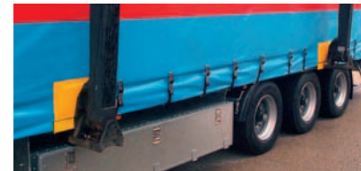
grapple pocket with correct marking
