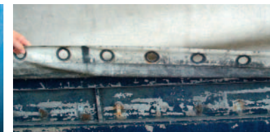
inadequately secured tarpaulin
