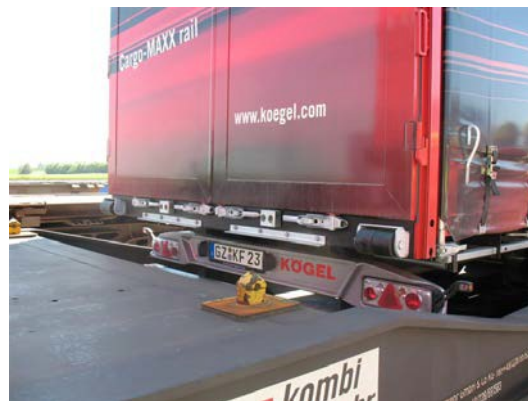
Left: 14.90 m semitrailer with retractable underride guard on pocket wagon T 3000. Right: 13.60 m semitrailer with fixed underride guard on pocket wagon T 3000. Picture credits: Kögel
