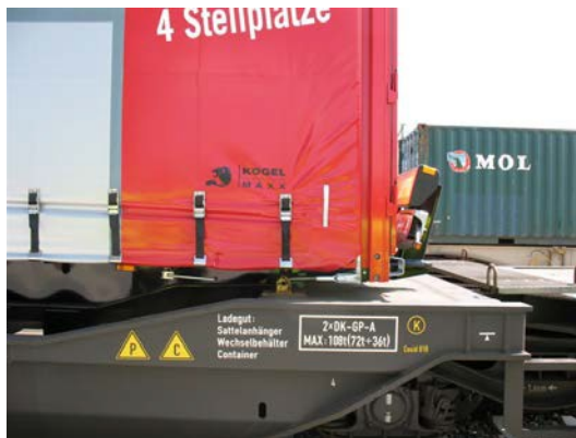
Left: 14.90 m semitrailer with retractable underride guard on pocket wagon T 3000. Right: 13.60 m semitrailer with fixed underride guard on pocket wagon T 3000. Picture credits: Kögel
